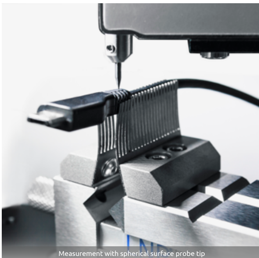
Multi-point measurement with 2 plastics and one rubber
