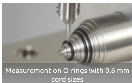
Young's modulus and hardness with s=30\mu\text{m}
